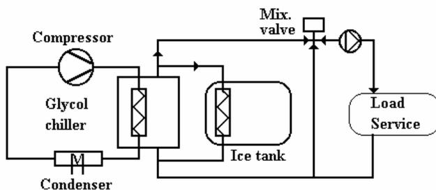
Figure 1. TES with internal melt system
