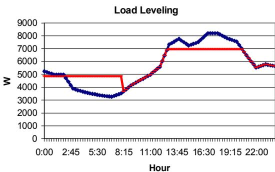
Figure 4. Load leveling and thermal loads
