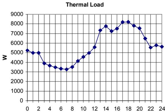
Figure 2. Thermal load for a residential customer
