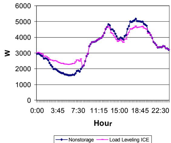
Figure 5. Effects of storage in customer load curve
